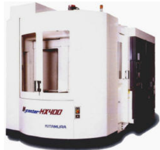
2006 Kitamura Pallet-type Horizontal Machining Center Model HX400iF
